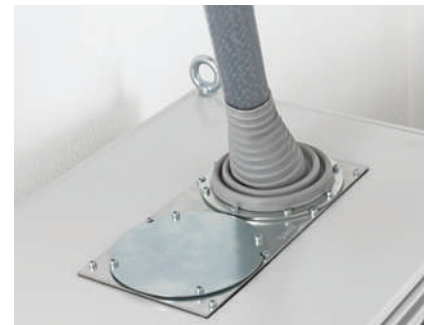
Routing of a rigid supply line through a closed enclosure roof via module plates. Cut-out size 314 x 144 mm.
